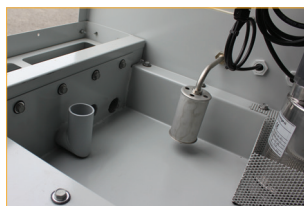
Fully drainable sump, accessible during operation
