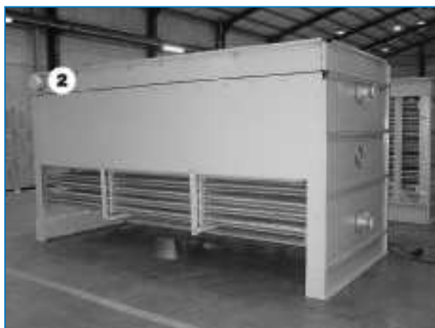
Pump piping connection on coil section
