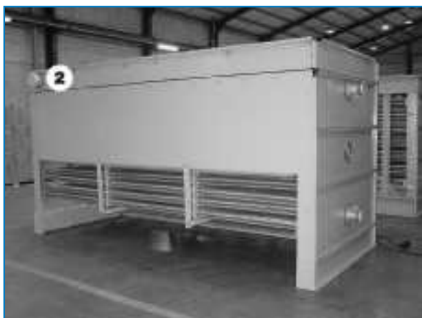
Pump piping connection on coil section
