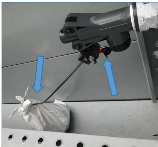
Fixation and wrapping of float ball
