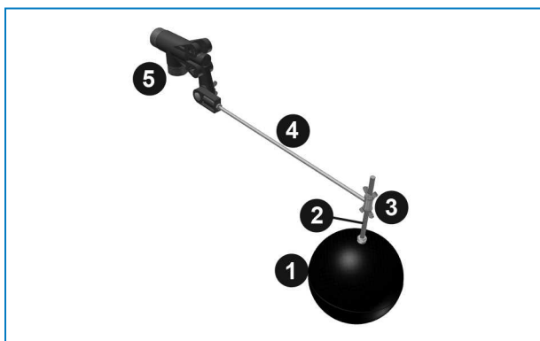
Water make-up valve assembly
