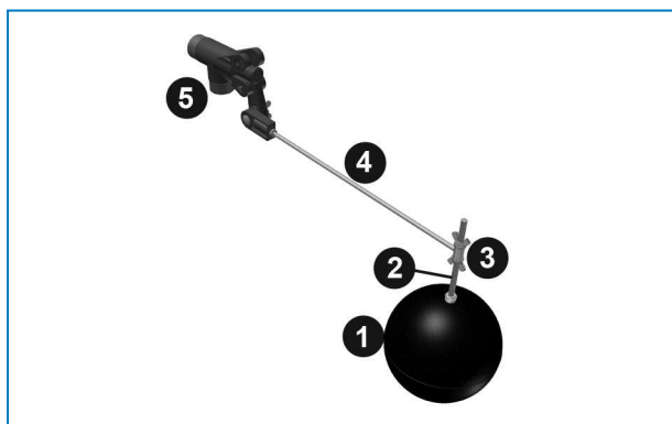
Water make-up valve assembly
